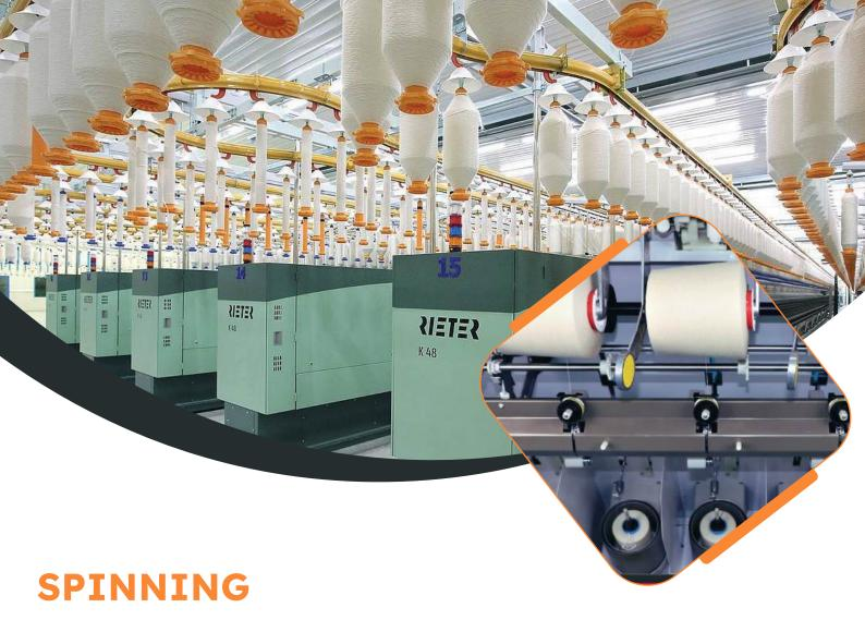
Our spinning division facilitates the production of the finest combed cotton yarn. While 50% of the facility is dedicated to manufacturing heavier count yarns like 30s, 34s & 40s, the remaining 50% produces finer yarn of counts 60s & 80s.
